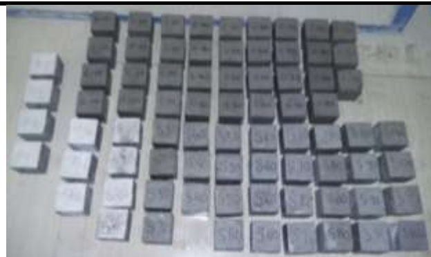
Fig.1: Mortar cubes prepared during experimental work for curing and compressive testing in the
